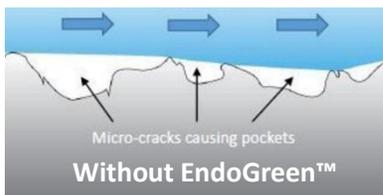
With the addition of **EndoGreen™** at the optimal concentration, the water hydrogen bonds are broken, thereby reducing the surface tension to as low as 27 mN/m, compared to 71 mN/m in untreated water. This alters the way steam bubbles form at the nucleated boiling sites along the imperfections found on the heating surfaces of fired boiler tubes.
